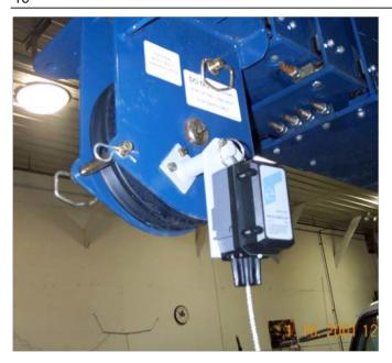
For jib installations, locate the switch close to the jib head.
