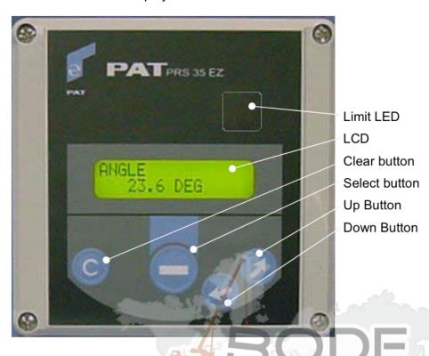
Fig 2: Operator's Console TECHNICAL SERVICES
